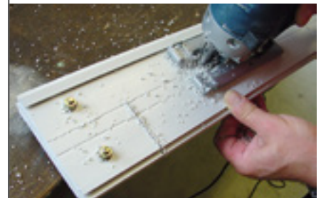
Cut the side panels to make the opening for inserting the wiring.
