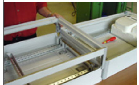
Refit the drilled and cut side panels, then replace the faceplate support frames
