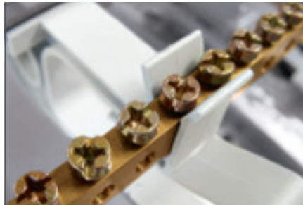
Horizontal wiring guide rings Cat.No 0 200 94 enable an additional brass collector Cat. No 0 373 00 to be installed between the rows.
