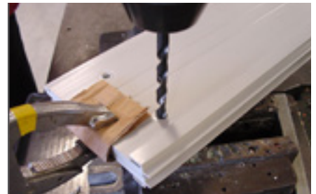
Drill both sides at the same time (Ø 6.5 mm)
