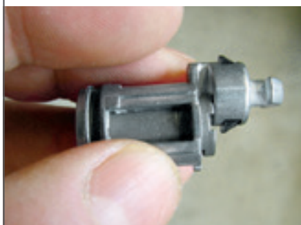
Combine the adaptor casing and barrel assembly with the aluminium-coloured adaptor
