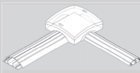
Application example for the floor-box, suitable for 90° branches or transitions from ABK 12x50 to 18x75
