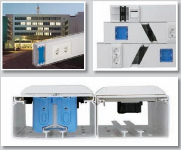
For both wall mounting and overhead (ceiling) mounting, the KHK holding clamps are simply inserted into the base (catch connection). During the fitting of the cables, the KHK holding clamps can easily be moved: Wherever space for the installation is needed, KHK holding can be positioned in order to create this space – without awkward grid perforation in the base.
