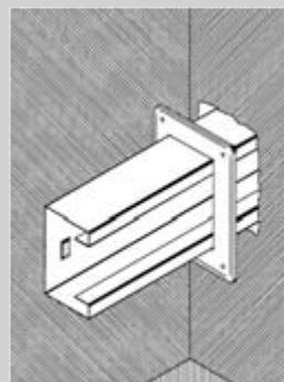
Wall connection panel for console mounting,
