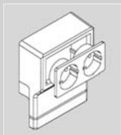
Device carrier systems, pre-wired, with height compensation either by using the included adapter or by breaking the bottom (break-off) edge
