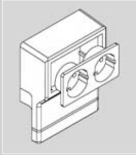
Device carrier systems, pre-wired, with height compensation either by using the included adapter or by breaking the bottom (break-off) edge
