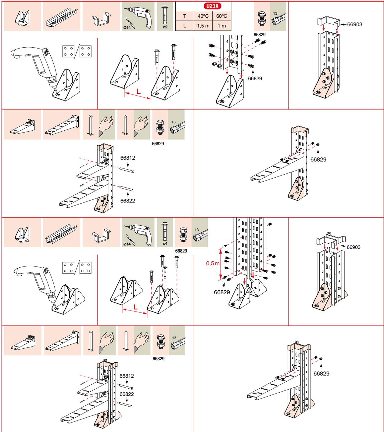
Note: The metal profiles should be painted in the unprotected areas when they are cut. (a) If a mounting pin is used, screws are not necessary to fix the horizontal support. (b) Join 2 profiles with 1 screws SST M8x25 part no. 66829 every 0,5 m.
