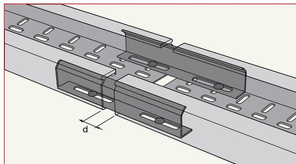
Coefficient of linear expansion: 0,07 mm/°C m
